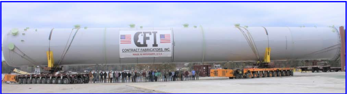
CONTRACT FABRICATORS, INC. CFI recently completed fabrication of a large pressure vessel that was shipped by water to an oil refinery in Louisiana. The gigantic vessel is 212 feet long by 15 feet in diameter and weighs over 400 tons. Photo was provided by Operations Manager Dustin Smith. You may learn more about CFI at www.contractfab.com .
